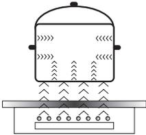
Electric oscillator powers a coil placed inside the appliance. This coil produces a magnetic field, which induces eddy currents in the cookware. These eddy currents induced by the magnetic field cause the cookware to heat up.
