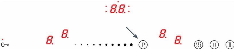
Booster function increases the power of the 220x190 mm cooking zone from 2200W to 3700W, and Bridge cooking zone (220 x 390 mm) from 3600W to 5500W.
