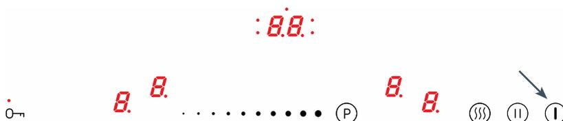
Touch and hold the on/off sensor for at least 1 second
