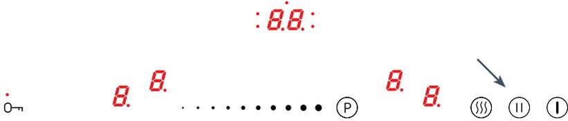
Stop'n go function acts like a pause. The Stop'n go function simultaneously suspends operation of all cooking zones and then resumes at the heat settings that were previously set. In order to activate the Stop'n go function, at least one cooking zone must be in use.
