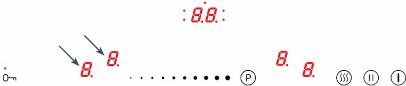
The Bridge function allows pairing of two cooking zones into a single combined cooking zone. The Bridge function is very convenient, especially when cooking in large pots such as a baking pan.
