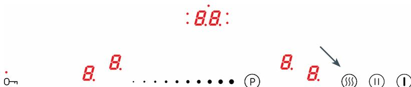
Keep warm function allows you to keep food warm on a cooking zone. The selected cooking zone operates at a low heat setting. With this feature, ready to serve, warm food retains its taste and does not stick to the pot's bottom. This function can be used to melt butter or chocolate.
