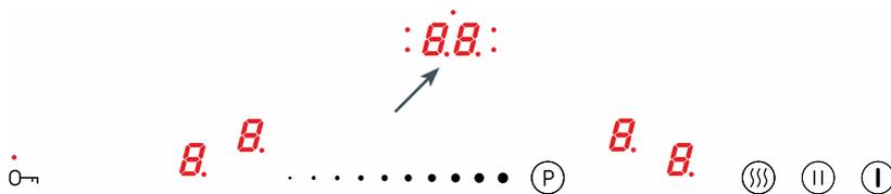
Timer function makes cooking easier by making it possible to set Duration. It can also be used as a Kitchen Timer. You can activate the Timer function only when cooking (when heat setting is greater than "0"). You can use the Timer function on all cooking zones at the same time. Maximum time is 99 minutes (1 minute step).
